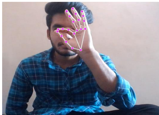
Figure 3. Click Operation using the Index and Thumb Fingers
