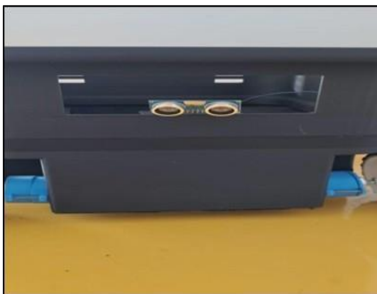
Figure 5. Ultrasonic Sensor Module Integrated into the Autonomous Delivery Robot for Obstacle Detection
