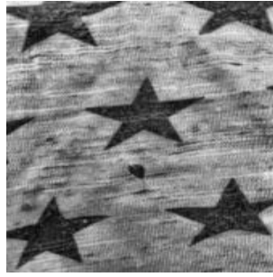
Figure 5 (a). Defected Image (hole)
