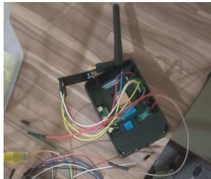
Figure 3.5. nRF24L01 Transceiver and Raspberry Pi Connection.
