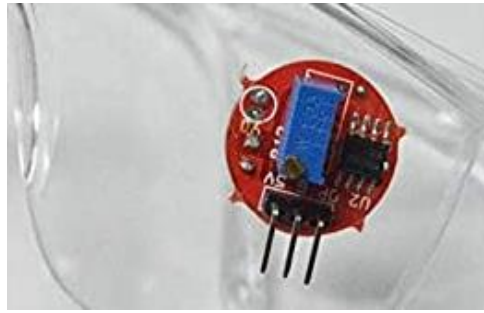
Figure 3.1. Eye Blink Sensor
