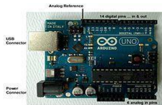
Figure 3.2. Arduino AT Mega 328
