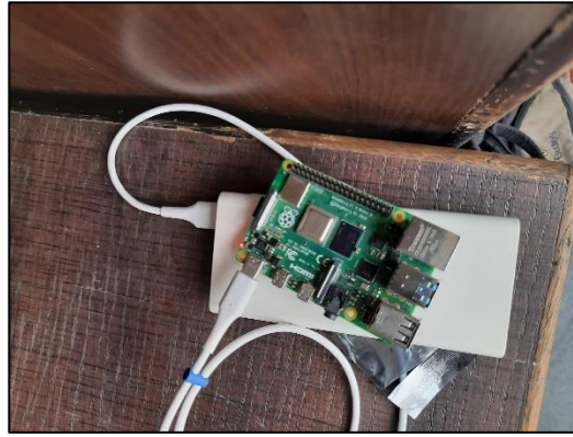
Figure 4. Raspberry Pi Server
