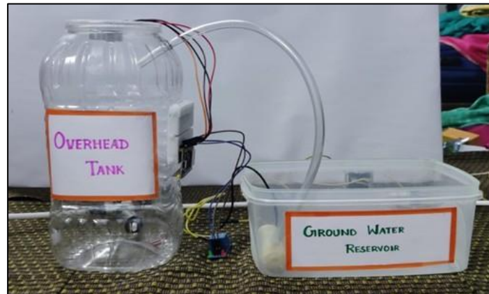
Figure 6. Hardware Setup for Overhead Tank
