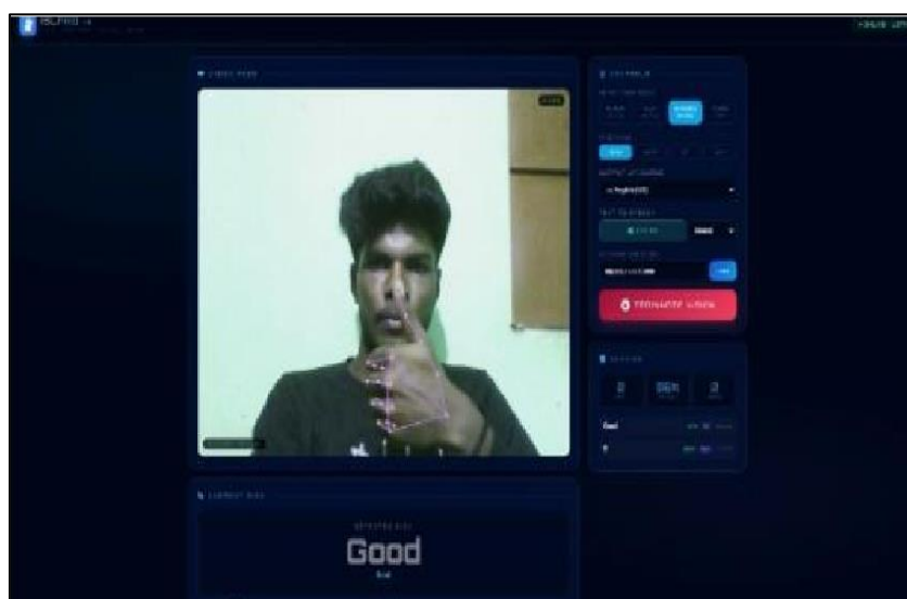
Figure 6. Recognition of the ISL Gesture Corresponding to the Word “Good”
