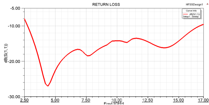
Figure 3. Return loss curve
