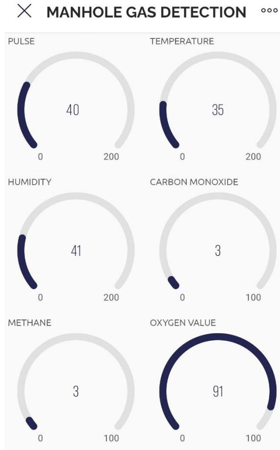
Fig 9. All sensor's data displayed in Blynk Application
