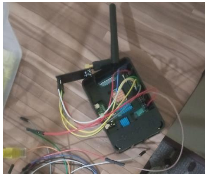
Figure 3.5. nRF24L01 Transceiver and Raspberry Pi Connection.
