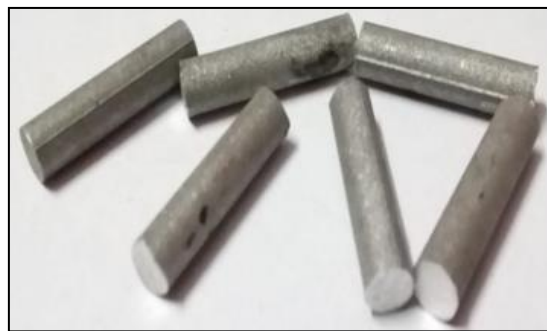
Figure 5. Specimen Before Compression
