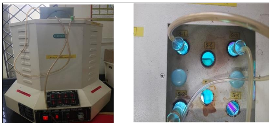
Figure 7. Experimental Setup of the Iron Nanomembrane–UV Photocatalytic Reactor Employed for Amoxicillin Degradation Studies
