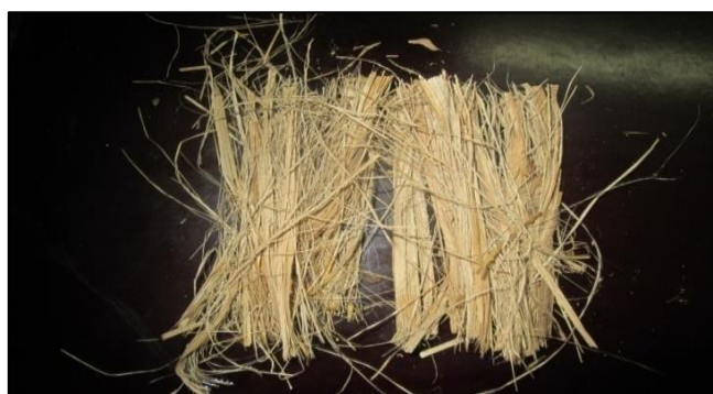
Figure 3. Alkali-Treated Banana Fibres after NaOH Surface Modification
