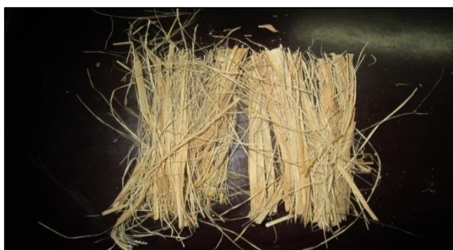
Figure 3. Alkali-Treated Banana Fibres after NaOH Surface Modification
