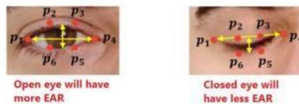
Figure 2. Eye Aspect Ratio [22]
