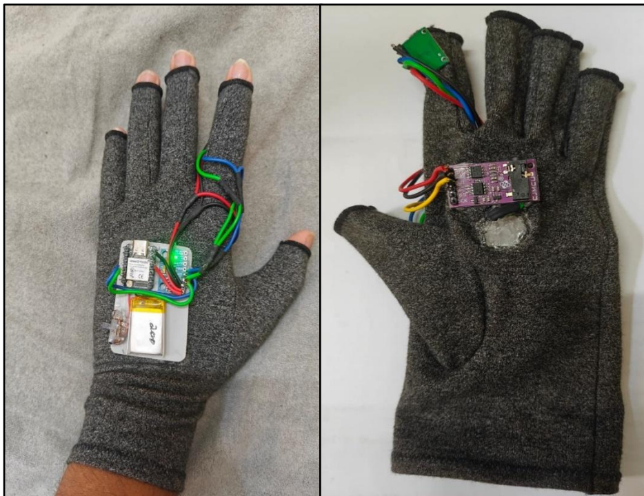
Figure 5. Telemetry Node (Wearable Smart Glove)
