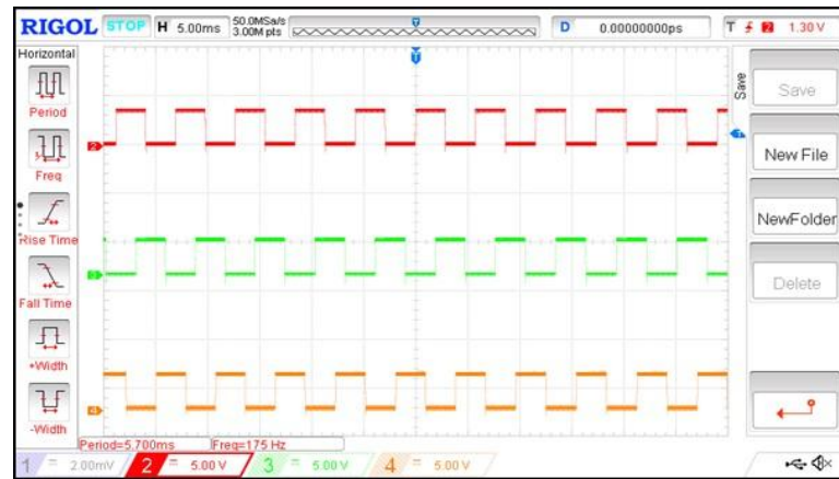
Figure 13. Hall Sensor Signals for 1500 rpm
