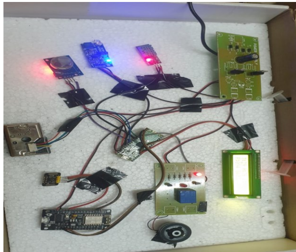
Figure 2. Final Representation of Gas Detection and Monitoring using RP2040 Controller
